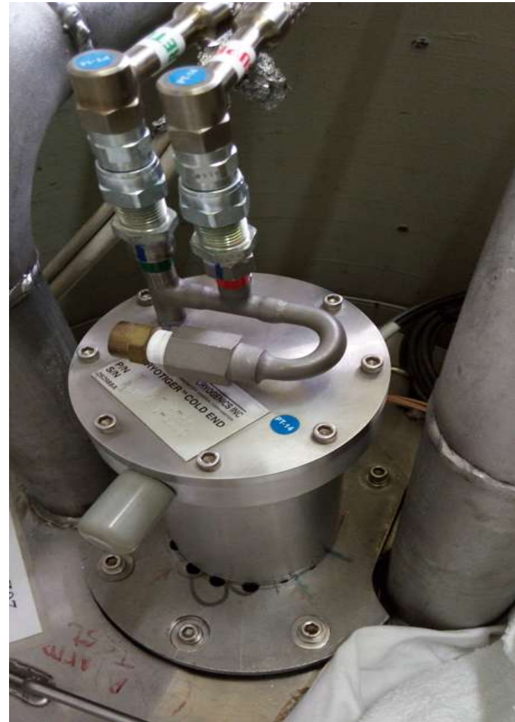
HPGe detector inside the Lead shield
