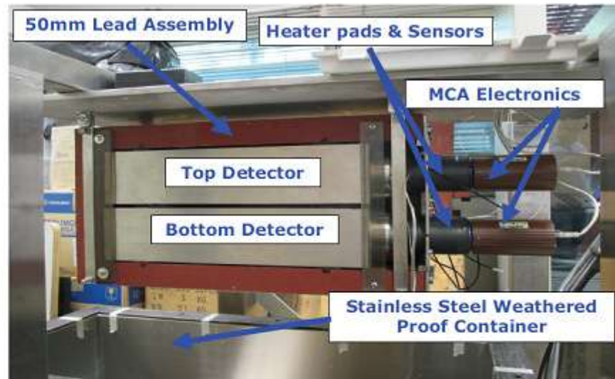
Detector, heaters, Lead Assembly & MCAs inside mobile cart
