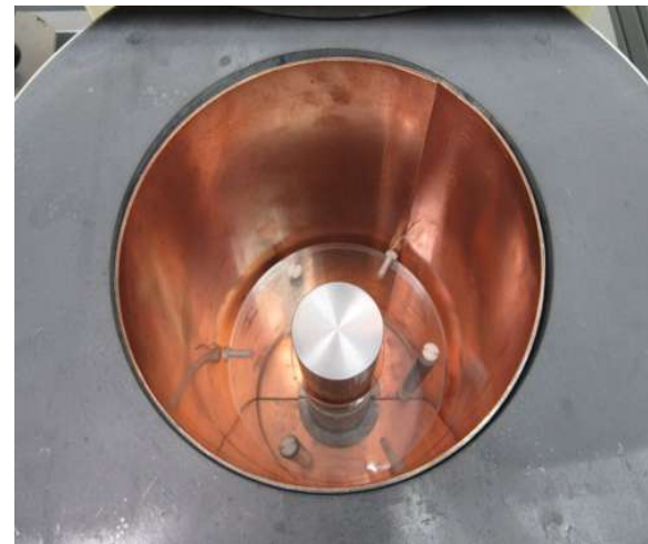
Detector inside Lead shield
